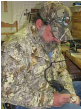
Above: Keith Hulm uses a rotary tool to route out the base of an antler that will eventually become a coyote call. Right: Hulm displays a finished call in his workshop.
