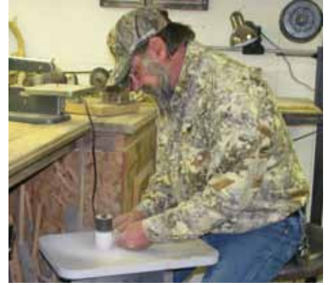
A drum sander helps shape the call's mouthpiece.
